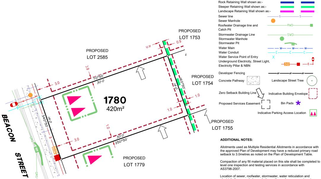
Location of sewer, rootwater, stormwater, water reticulation and electricity lines, manholes and pits are those shown on engineering design drawings, supplied by Peak Urban and may differ from the as-constructed location.
