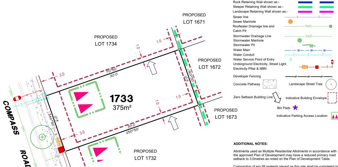
Compaction of any fill material placed on this site shall be completed to level one inspection and testing services in accordance with AS3798-2007.
