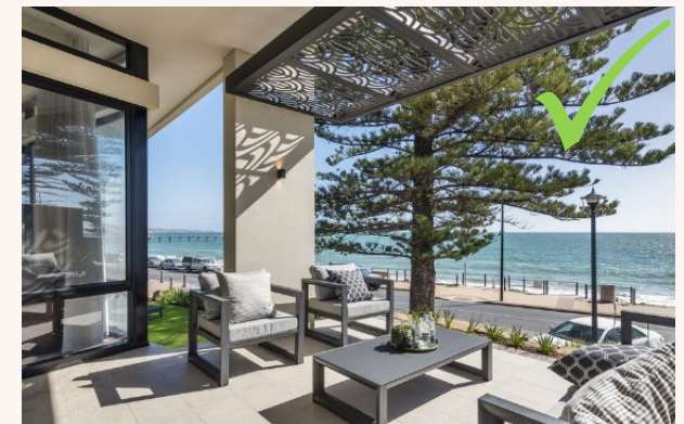
Projections up to 600mm forward of the main elevation are acceptable to provide articulation.
