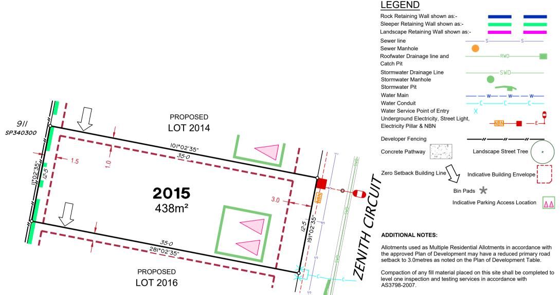
Location of sewer, roofwater, stormwater, water reticulation and electricity lines, manholes and pits are those shown on engineering design drawings, supplied by Peak Urban and may differ from the as-constructed location.
